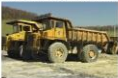
Figure 1. Even when empty, haul trucks can weigh 50 - 100 tons or more; this weight exerts force where tires meet the land surface, causing severe compaction of mine soils. Loaders, dozers, and other heavy mining equipment also cause compaction that hinders tree growth when operated on surface soils.
